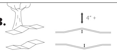
A deviation from the design or construction grade equal to 4" in a ten-foot section
